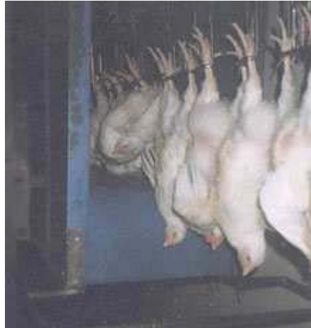
Figure 4: The poultry slaughter line before the vat where electronarcosis occurs, where one notices the way in which a bird can avoid electrification ( www.islamonline.net )
